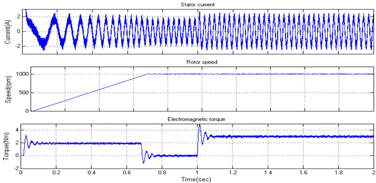
**Figure 6: Simulation result of basic 6-sector DTC showing current, speed, and torque**
