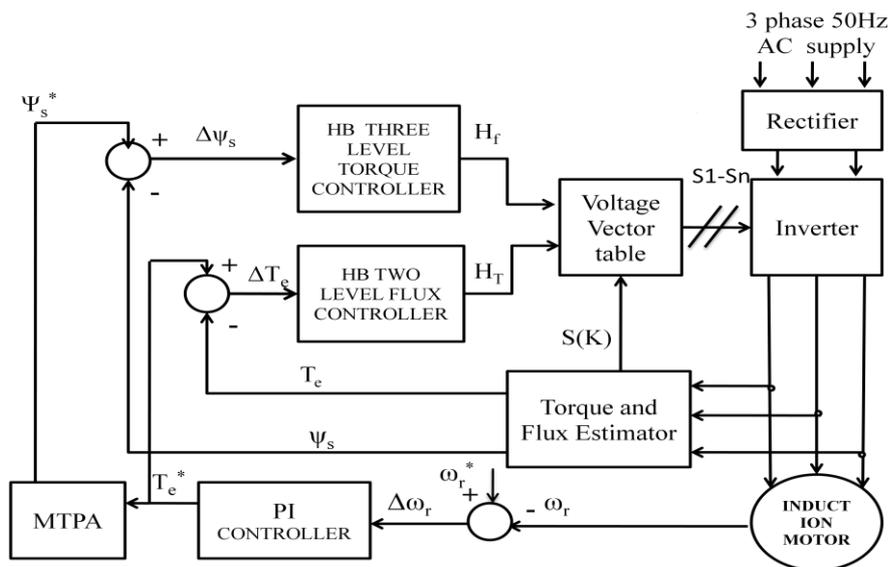
Figure 3: Block diagram of DTC for induction motor
