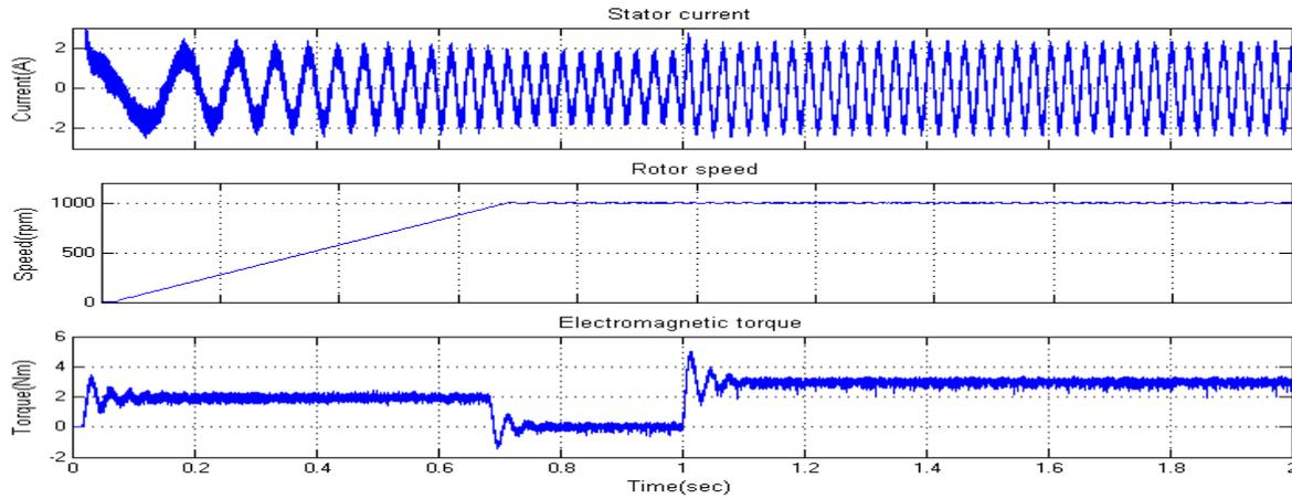
**Figure 5: Simulation result of basic 6-sector DTC showing current, speed, and torque**
