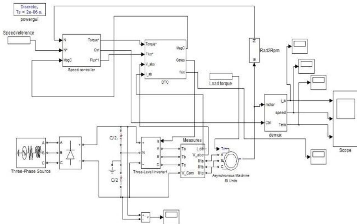
Figure 4: Simulation model of proposed 12-sector DTC
