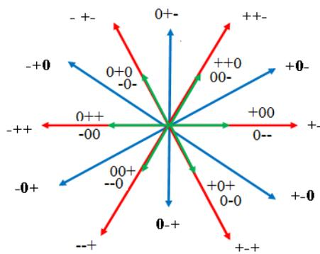
Figure 2: Switching state vectors of 3-level inverter
