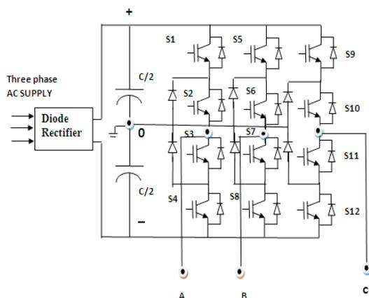
Figure 1: Neutral point clamped inverter
